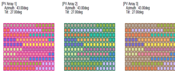
Fig. 8. Wiring for PV circuit
